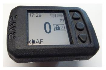
Your RAVE altimeter comes with a set of default parameters, please configure it before using it for skydiving activities according to your needs: language, alarm intensity, altitude trigger levels, metric vs. imperial measurement units, etc. Refer to the chapter 4. Menu for details.
